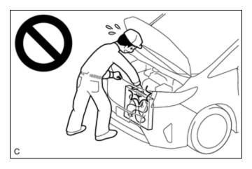
(a) Check the operation of the cooling fan while operating it using the GTS.
