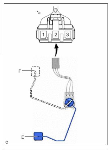
\*a Component without harness connected (Fuel Sender Gauge Assembly)
