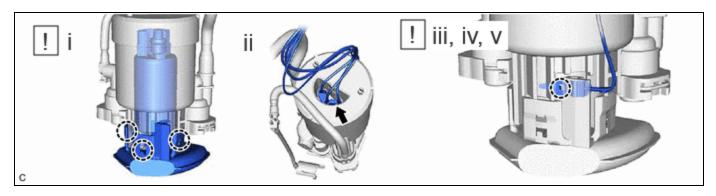
(1) Engage the 3 claws to install the fuel pump with filter assembly to the fuel filter.
