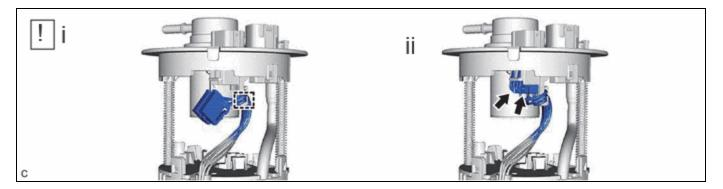
(1) Engage the clamp to connect the fuel pump harness to the fuel suction plate sub-assembly.
