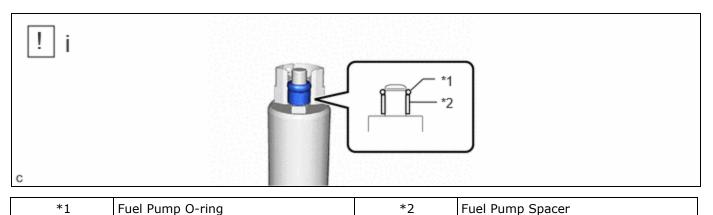
(1) Apply gasoline to a new fuel pump O-ring. Then install the fuel pump O-ring and fuel pump spacer to the fuel pump with filter assembly.
