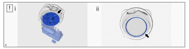
(1) Remove the fuel suction tube with pump and gauge assembly from the fuel tank sub-assembly.
