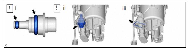
(1) Apply gasoline to 2 new O-rings. Then install the O-rings to the fuel main valve assembly.
