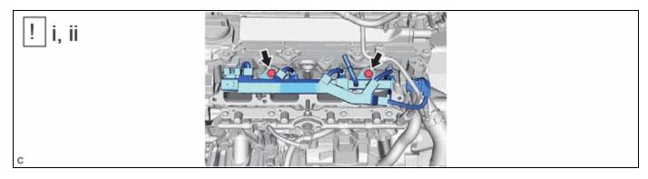
(1) Place the fuel delivery pipe sub-assembly with the 4 port fuel injector assemblies onto the cylinder head sub-assembly.
