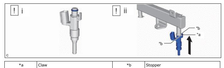
(1) Apply a light coat of spindle oil or gasoline to 4 new O-rings, and install one to each port fuel injector assembly.
