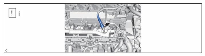
(1) Connect the fuel tube sub-assembly to the fuel delivery pipe sub-assembly.
