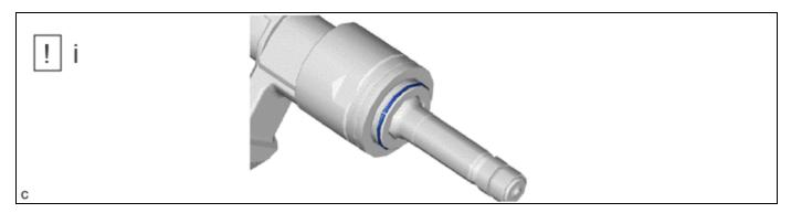
(1) Install a new C-ring to each direct fuel injector assembly.
