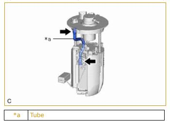
When replacing the fuel filter, replace it together with the fuel suction plate sub-assembly.
