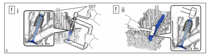
(1) Using SST, install the 16 valve spring retainer locks.
