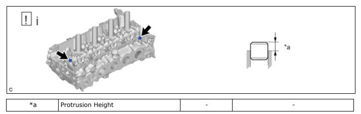
(1) Using a plastic hammer, tap in 2 new ring pins to the cylinder head sub-assembly.
