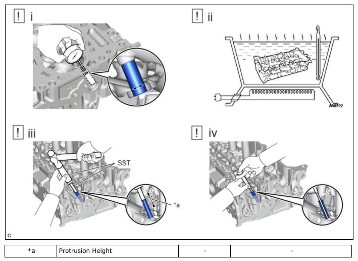
(1) Using a caliper gauge, measure the exhaust valve guide bush bore diameter of the cylinder head subassembly.
