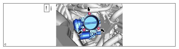
(1) Using an 8 mm socket wrench, install the throttle body with motor assembly to the intake manifold with the 3 bolts.
