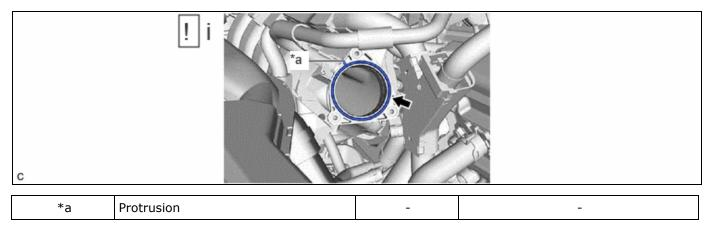
(1) Install a new throttle body gasket to the intake manifold with the protrusion of the throttle body gasket oriented as shown in the illustration.
