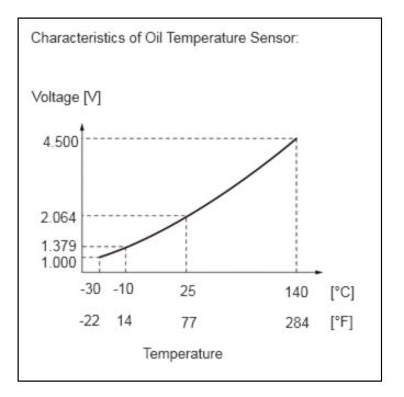
The engine oil temperature sensor (oil pressure and temperature sensor) replaces the oil temperature with electrical signals and outputs them to the ECM.
