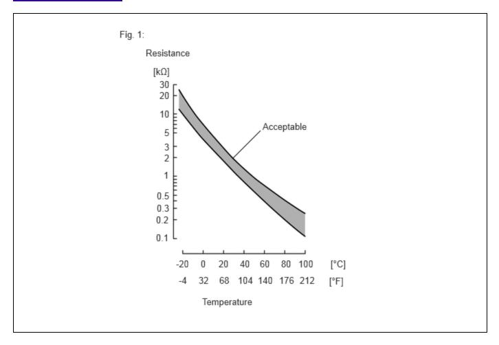
A thermistor, whose resistance value varies according to the engine coolant temperature, is built into the engine coolant temperature sensor. The structure of the sensor and its connection to the ECM are the same as those of the intake air temperature sensor.
