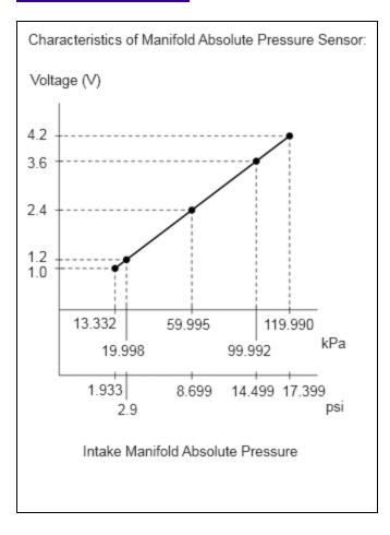
The manifold absolute pressure sensor detects the intake manifold pressure as a change in voltage. The ECM calculates the intake manifold pressure based on this voltage. The ECM calculates the EGR valve assembly and purge VSV opening amount according to changes in the intake manifold pressure and also detects malfunctions of the manifold absolute pressure sensor using these changes in pressure.
