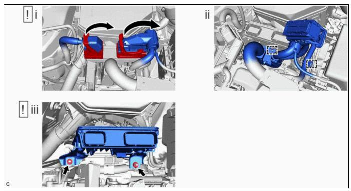
(1) Raise the 2 lock levers while pushing the locks on the levers, and disconnect the 2 ECM connectors.
