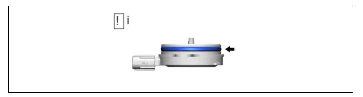
(1) Remove the cam timing oil control solenoid O-ring from the cam timing oil control solenoid assembly.
