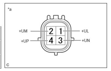
\*a (Fuel Vapor Containment Valve (Close Tank with Bolt Valve Assembly))
