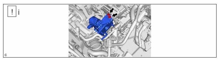
(1) Using the 8 mm socket wrench, remove the 2 bolts and EGR valve assembly.
