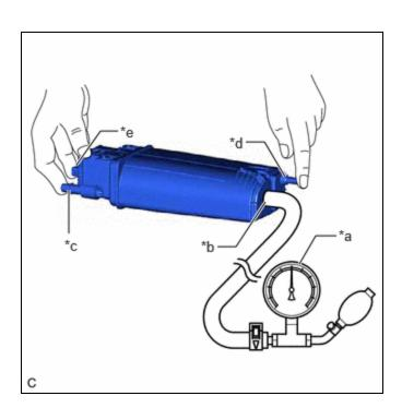
(a) Connect a pressure gauge to the vent line port.
