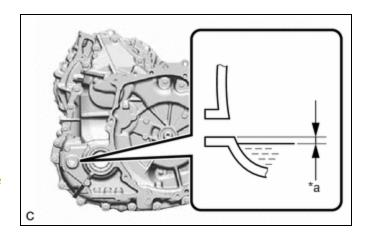
recheck the hybrid transaxle fluid level after driving the vehicle.
