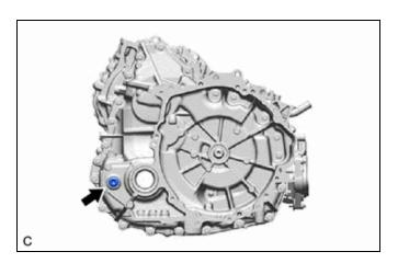
(b) Using a 10 mm hexagon socket wrench, remove the drain plug and gasket from the hybrid vehicle transaxle assembly and drain the hybrid transaxle fluid.
