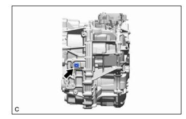
(c) Using a 10 mm hexagon socket wrench, install the drain plug and a new gasket to the hybrid vehicle transaxle assembly.
