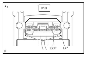
\*a (Shift Control ECU (Transmission Floor Shift Assembly))
