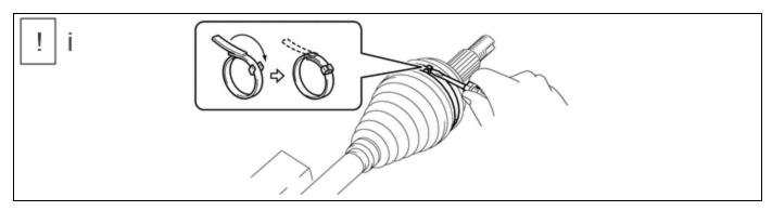
(1) Using a screwdriver, install the rear No. 2 drive shaft outboard joint boot clamp as shown in the illustration.
