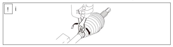
(1) Using pliers, separate the rear drive shaft outboard joint boot clamp as shown in the illustration.
