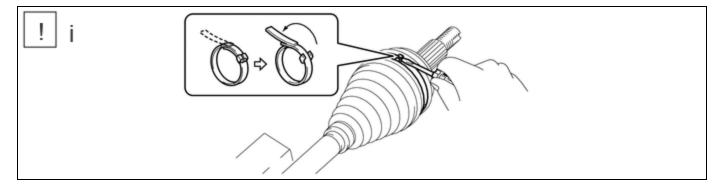
(1) Using a screwdriver, separate the rear No. 2 drive shaft outboard joint boot clamp as shown in the illustration.
