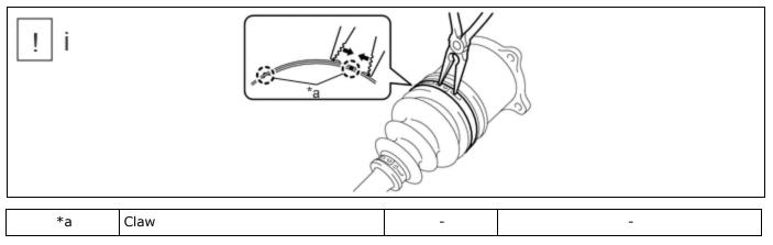
(1) Using needle-nose pliers, disengage the 2 claws as shown in the illustration and separate the rear No. 2 drive shaft inboard joint boot clamp.
