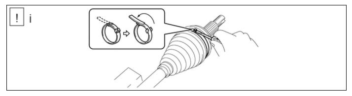
(1) Using a screwdriver, release the staked part of the front No. 2 axle outboard joint boot clamp and separate the front No. 2 axle outboard joint boot clamp.
