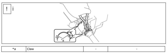
(1) Using needle-nose pliers, separate the 2 front drive shaft damper clamps.
