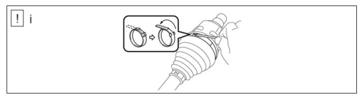
(1) Using a screwdriver, release the staked part of the front No. 2 axle inboard joint boot clamp and separate the front No. 2 axle inboard joint boot clamp.
