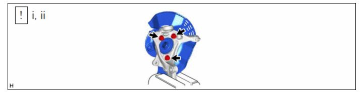
(1) Secure the steering knuckle between aluminum plates in a vise.
