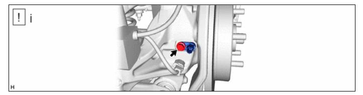
(1) Remove the bolt and the rear skid control sensor from the rear axle carrier sub-assembly.
