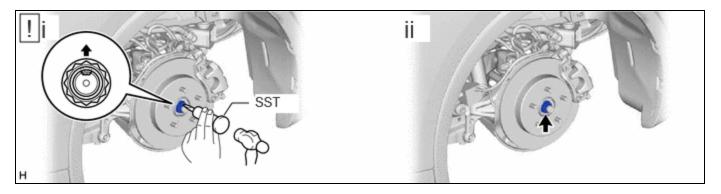
(1) Using SST and a hammer, release the staked part of the rear axle shaft nut.
