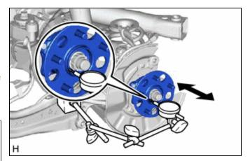
(b) If the looseness exceeds the maximum, replace the rear axle hub and bearing assembly.
