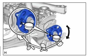
(b) If the runout exceeds the maximum, replace the rear axle hub and bearing assembly.
