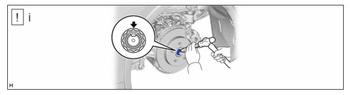
(1) Using a chisel and hammer, stake the rear axle shaft nut.
