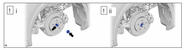
(1) Clean the threaded parts on the rear drive shaft assembly and a new rear axle shaft nut using non-residue solvent.
