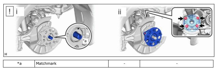
(1) Install the rear axle hub and bearing assembly and rear disc brake dust cover sub-assembly to the rear drive shaft assembly.
