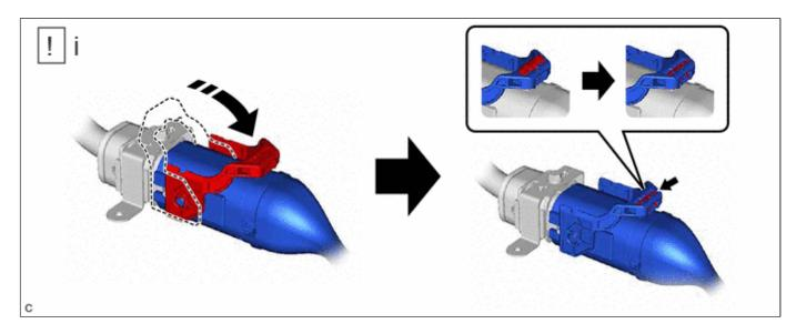
(1) Connect the rear traction motor cable connector.
