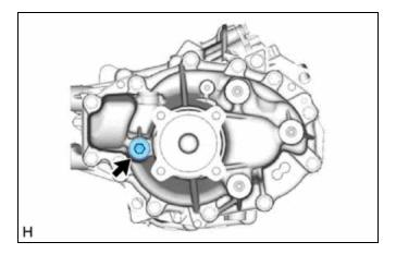
(b) Add hybrid transaxle fluid until the hybrid transaxle fluid level is between 0 to 5 mm (0 to 0.197 in.) from the bottom lip of the filler plug opening. [#]
