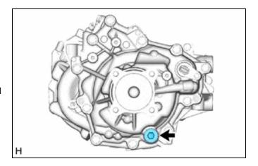
(c) Using a 10 mm hexagon socket wrench, install a new gasket and the drain plug to the rear traction motor with transaxle assembly.
