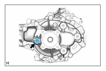
(b) Using a 10 mm hexagon socket wrench, remove the drain plug and gasket from the rear traction motor with transaxle assembly and drain the hybrid transaxle fluid.
