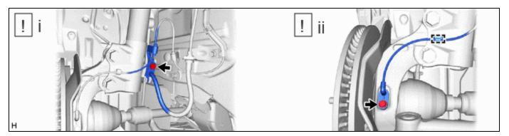
(1) Remove the bolt and separate the front speed sensor and front flexible hose from the front shock absorber assembly.
