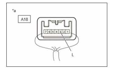
\*a Component with harness connected (Stop Light Switch Assembly)
