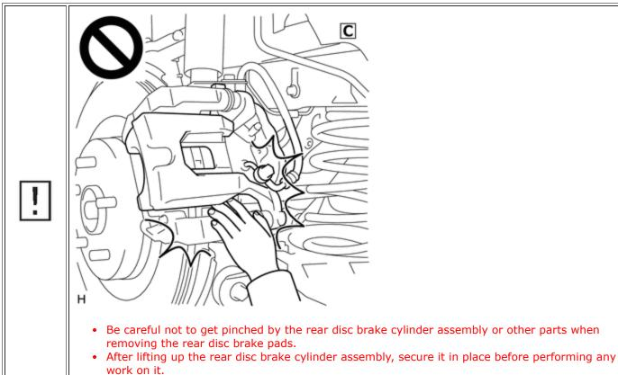
The rear disc brake cylinder assembly could fall, pinching hands or fingers and causing injury.
