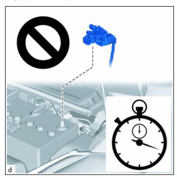
(c) Before starting work relating to the SRS airbag system, fitting adjustment of the front/rear doors and removal, installation or replacement of parts near the airbag sensors, wait for at least 60 seconds after disconnecting the cable from the negative (-) auxiliary battery terminal.
