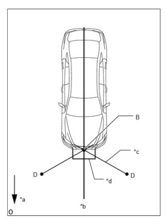
(7) Align a piece of string with line C and mark point D at a distance of 3088 mm (10.13 ft.) from point B.
