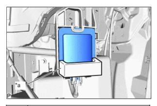
\*a SST (Digital Angle Gauge Attachment A)
