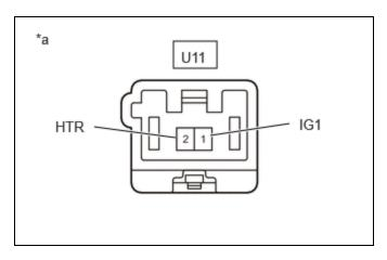
\*a Component without harness connected (Windshield Glass (Heater))
