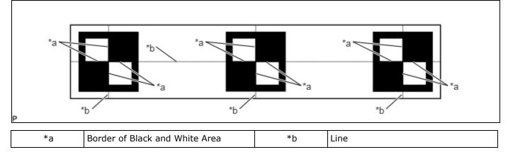
(5) Securely attach the target sheets to the cardboard using double-sided tape.
