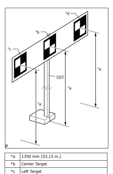
(e) Prepare an object to block the area behind the target. (If there are any objects which may be misrecognized as a target behind the area where a target will be placed.)
