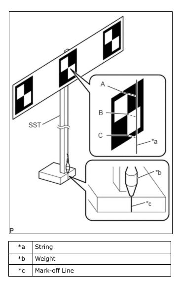
(d) Move SST (reflector) up or down so that the center of the 3 target sheets is at the height shown in the illustration, and secure SST (reflector) in place.
