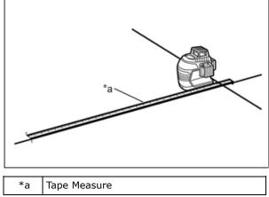
6. At a distance of 3000 mm (9.84 ft.) from point B, apply an approximately 200 mm (7.87 in.) piece of tape
