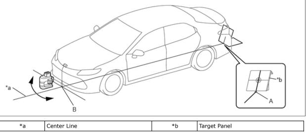
4. Adjust the position of the laser line marker so that the laser beam is aligned with the center line of the target panel.
