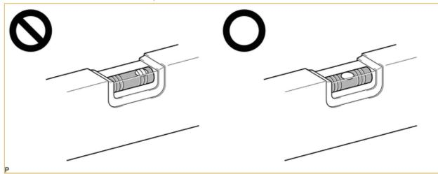
(c) Perform Front Beam Axis Adjustment.
