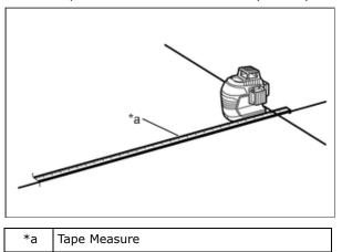
6. Mark point C at a distance of 1500 mm (4.92 ft.) from point B, and apply a 300 mm (11.81 in.) piece of tape alongside the tape measure so that the tape extends 150 mm (5.91 in.) to the front and rear of point C.
