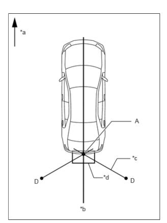
(7) Align a piece of string with line C and mark point D at a distance of 2838 mm (9.31 ft.) from point A.
