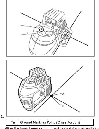
Align the laser beam ground marking point (cross portion) with point A.
