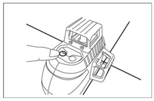
2. Adjust the position of the laser line marker so that the laser beam passes through point C and point D as shown in
