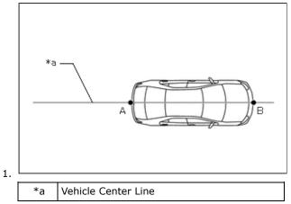
Draw a vehicle center line so that it passes through mark A and B (front and rear center points).
