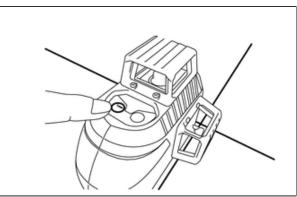
2. Align the laser beam ground marking point (cross portion) with point B.
