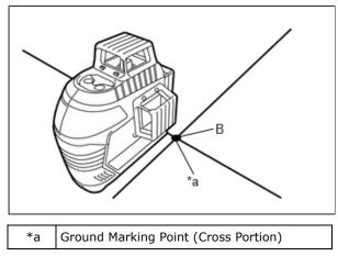
ADVANCED DRIVER ASSISTANCE SYSTEM: MILLIMETER WAVE RADAR SENSOR: TARGET ADJUSTMENT(TRIANGLE TARG...
