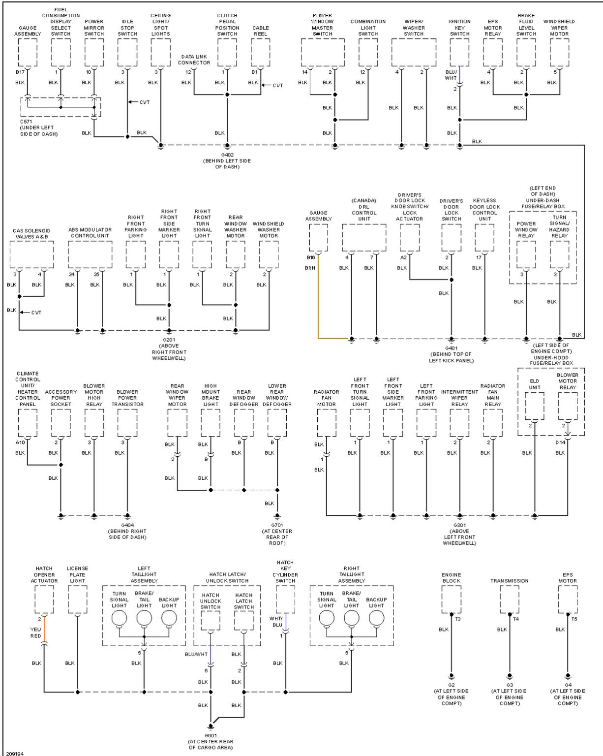
**Fig. 24: Ground Distribution Circuit (2 of 2)**
