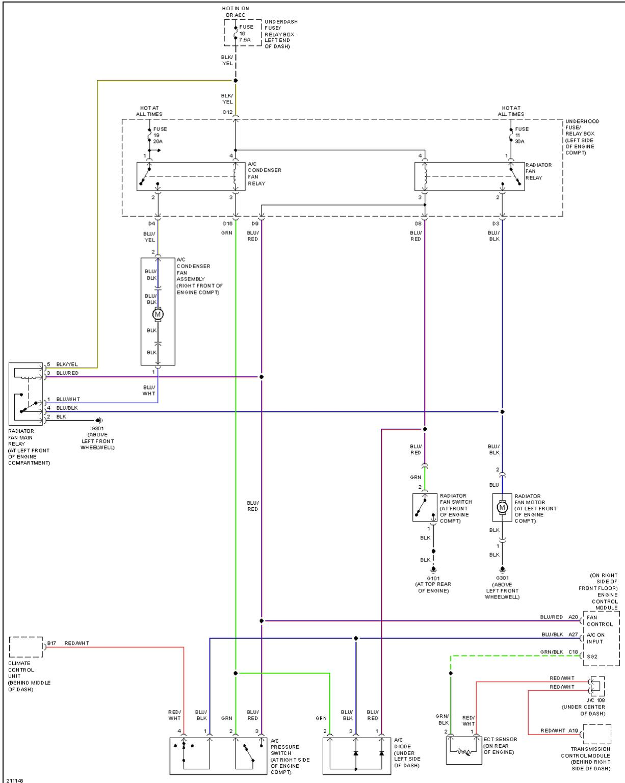
**Fig. 7: Cooling Fan Circuit, W/ A/C**
