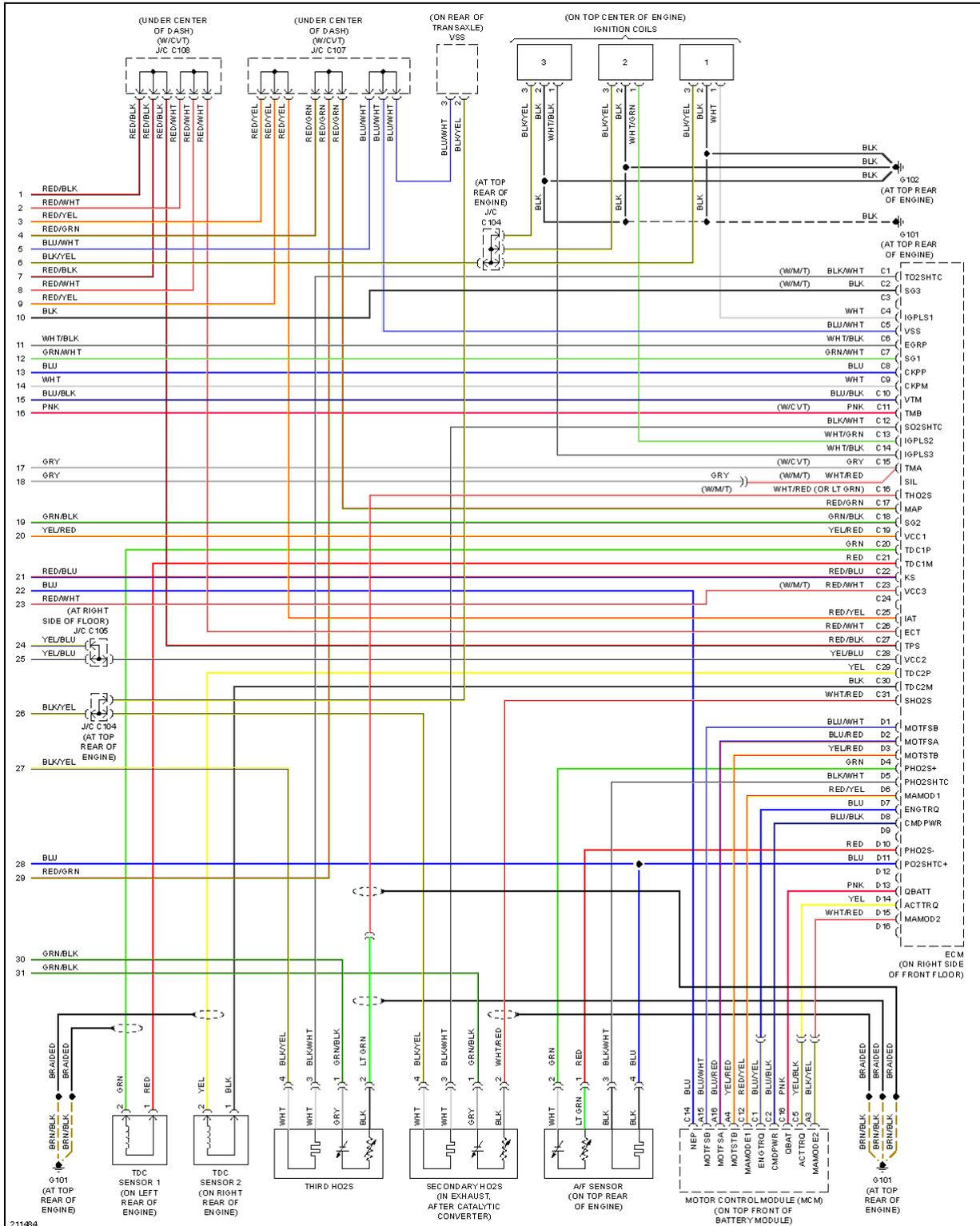
**Fig. 19: 1.0L, Engine Controls Circuit (4 of 4)**
