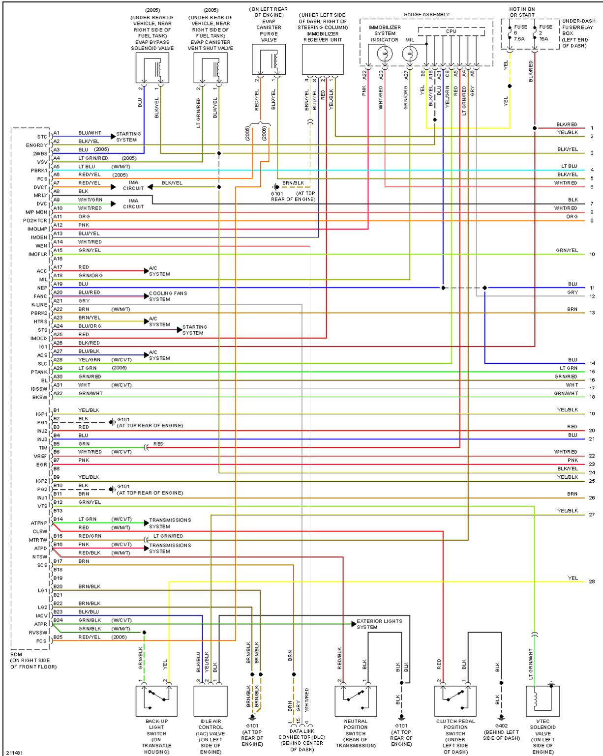
**Fig. 16: 1.0L, Engine Controls Circuit (1 of 4)**
