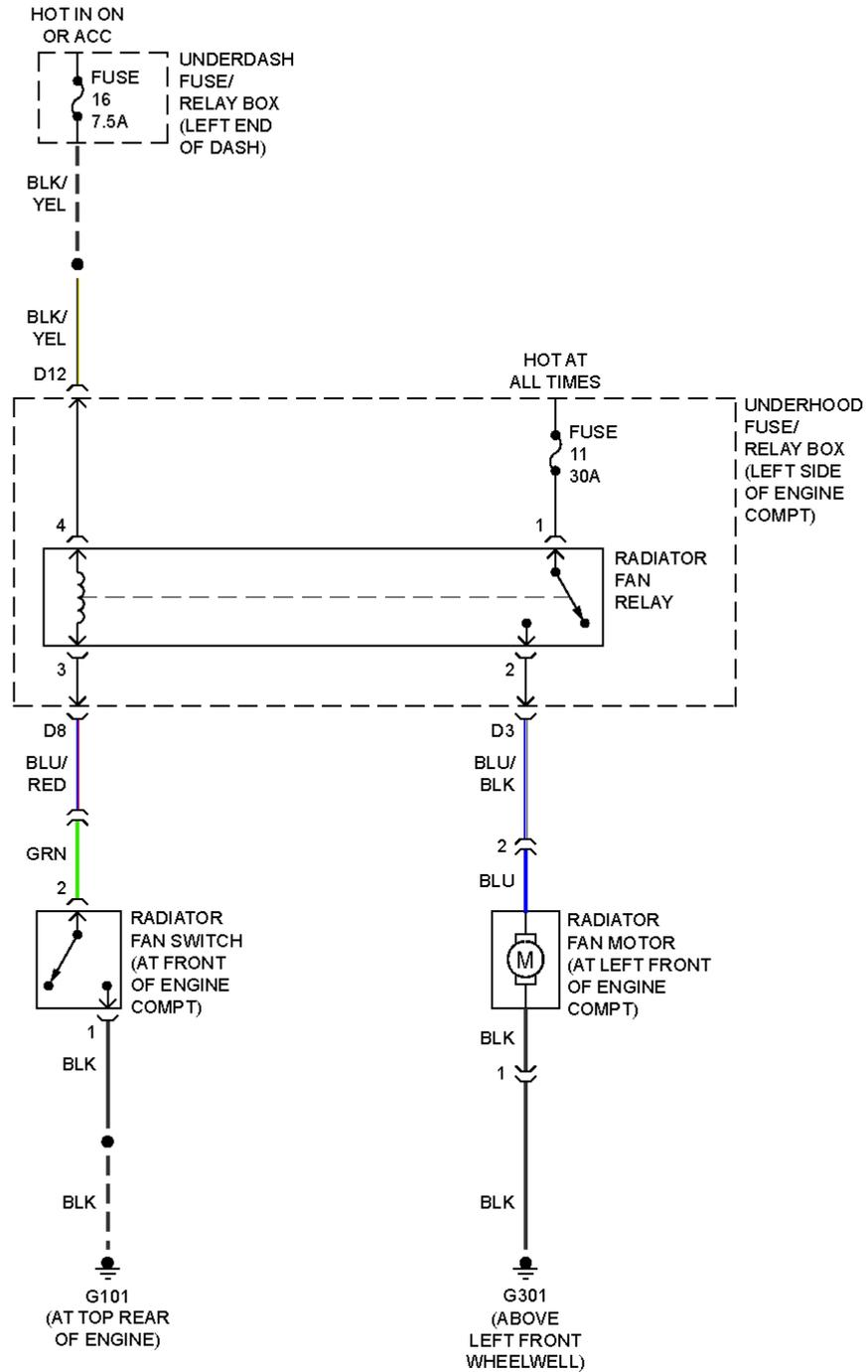
**Fig. 8: Cooling Fan Circuit, W/O A/C**
