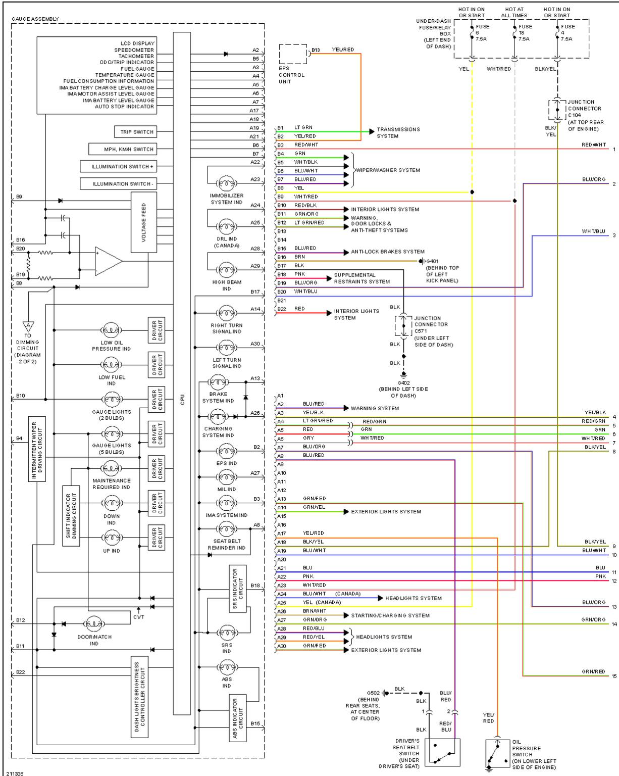
**Fig. 28: Instrument Cluster Circuit (1 of 2)**
