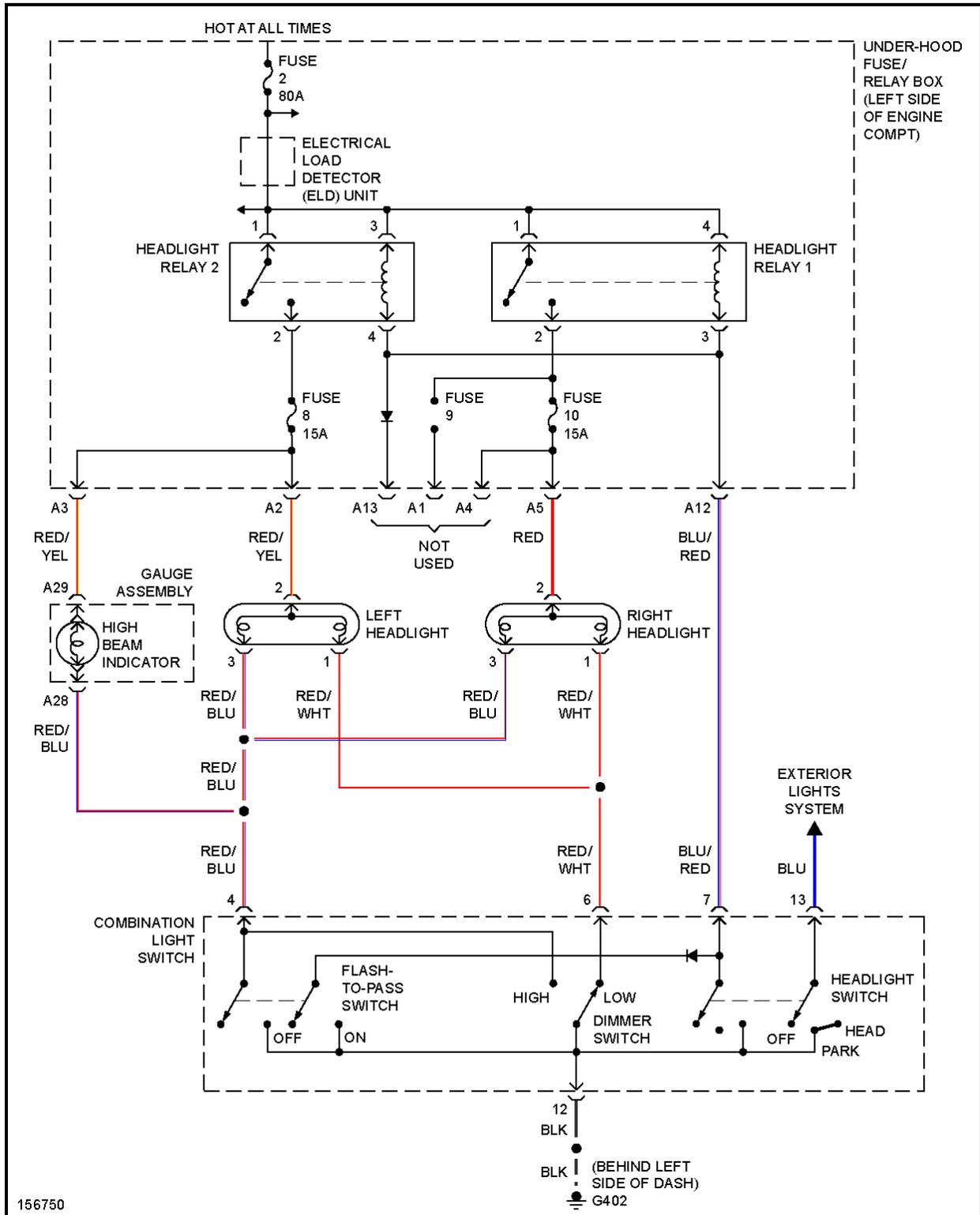
**Fig. 26: Headlights Circuit, W/O DRL**
