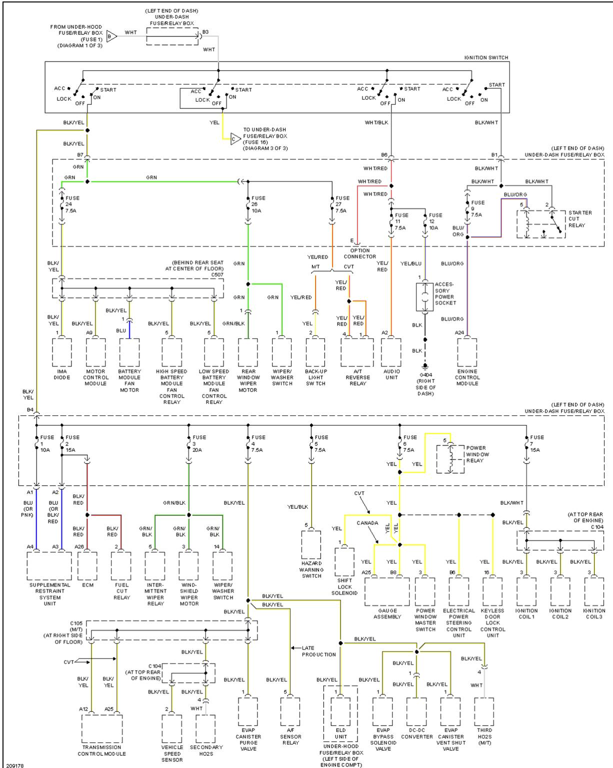
**Fig. 33: Power Distribution Circuit (2 of 3)**
