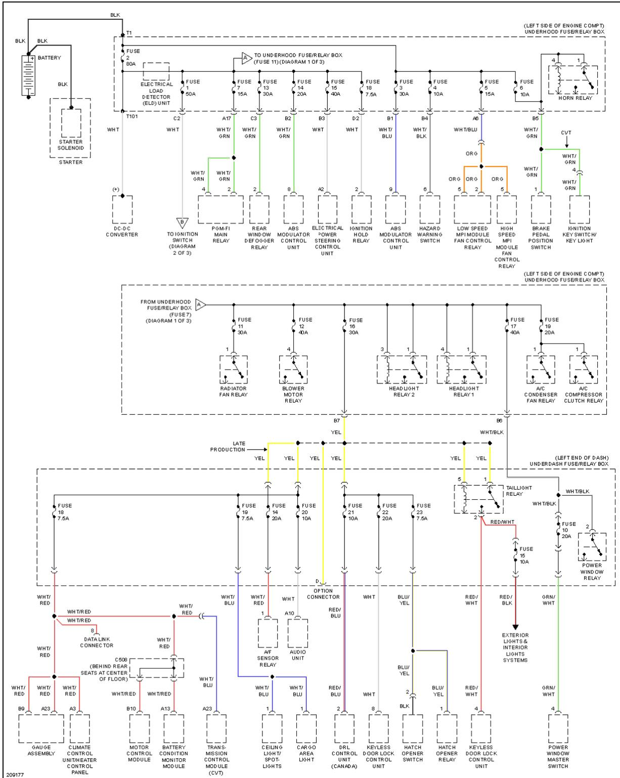
**Fig. 32: Power Distribution Circuit (1 of 3)**
