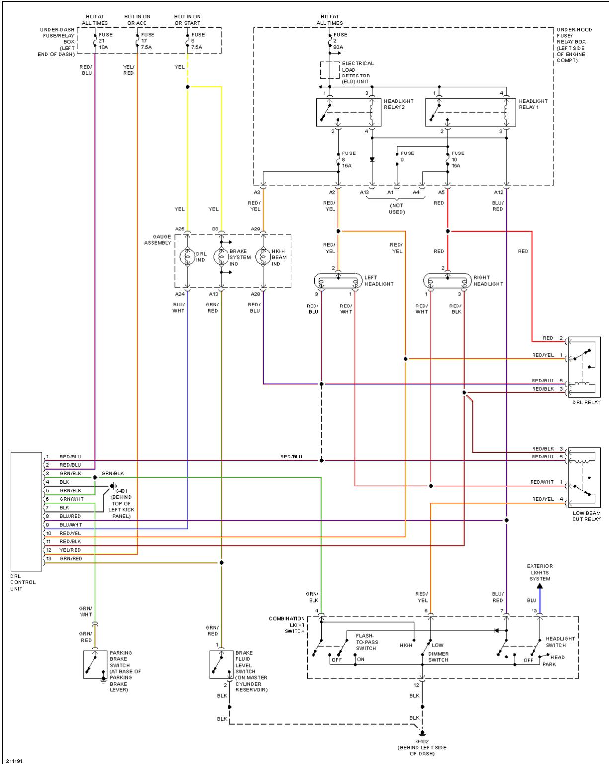
**Fig. 25: Headlights Circuit, W/ DRL**
