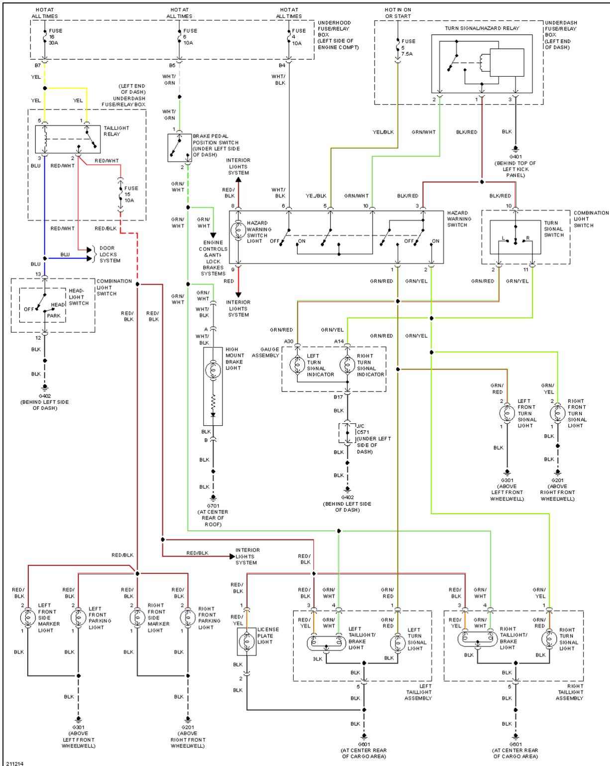
**Fig. 22: Exterior Lamps Circuit**
