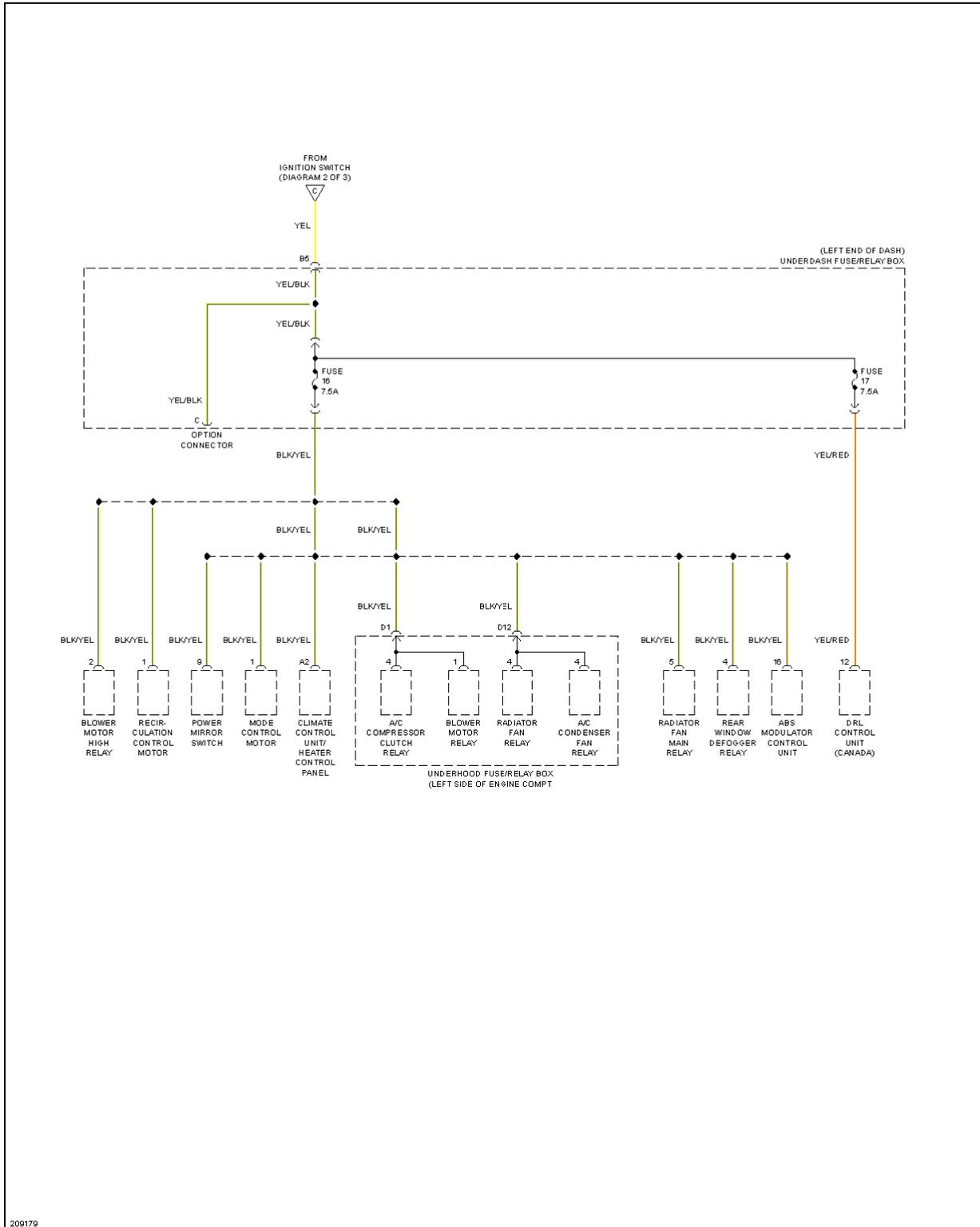
**Fig. 34: Power Distribution Circuit (3 of 3)**
