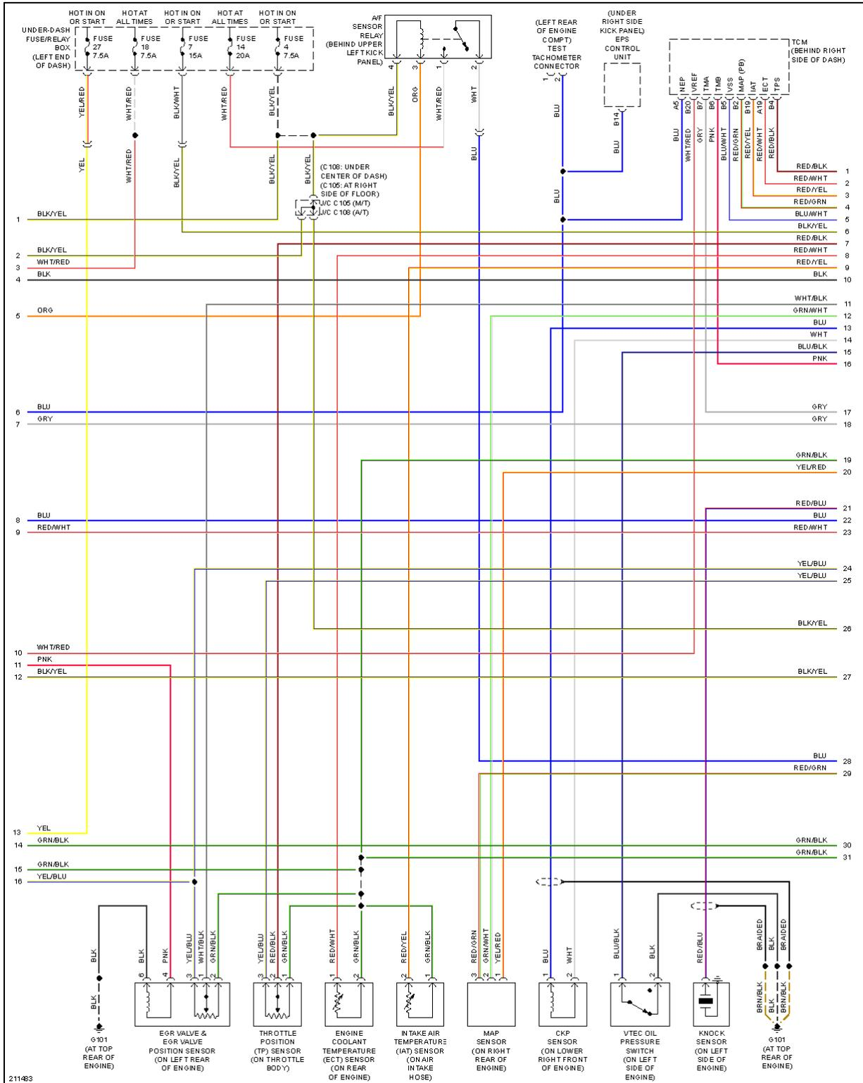
**Fig. 18: 1.0L, Engine Controls Circuit (3 of 4)**
