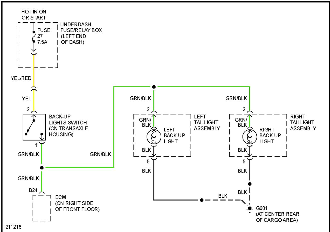
**Fig. 21: Back-up Lamps Circuit, M/T**
