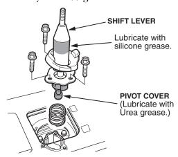
• Lubricate the shift lever with silicone grease as shown. This keeps it from squeaking as it rubs against the shift boot.
