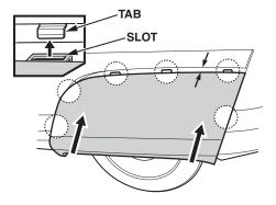
2. Install the two stud fasteners. Turn each fastener **180 degrees**, no more. (You know you've done it right when the small, round dot on the skirt lines up with the arrow on the fastener.)
