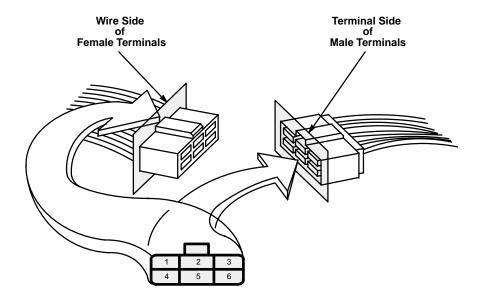
The connector cavity number is listed next to each terminal on the circuit schematic. The cavity/terminal shown below is #6.
