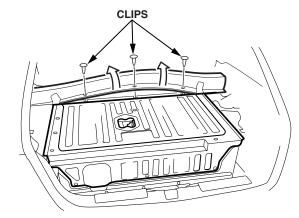
7. Remove the under-cover (two bolts, two clips, and three screw clips).
