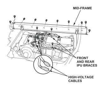
12. Disconnect the high-voltage cables from the output terminals on the junction board, and wrap them with insulating tape.
