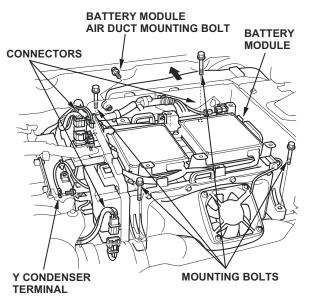
14. Remove the mounting bolts from the battery module. Disconnect the connectors and the Y condenser terminal.
