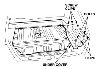
8. Remove the IPU (intelligent power unit) lid (six Torx bolts and 17 hex bolts).
