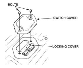
4. Flip the battery module switch to OFF, then reinstall the locking cover.
