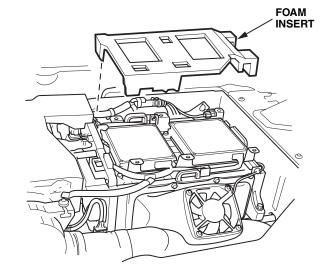
11. Remove the mid-frame, then remove the front and rear IPU braces from the junction board.
