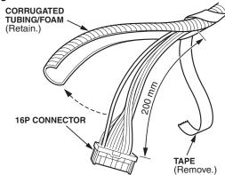
10. Locate the RED/WHT wire in the 16P connector. Then measure 150 mm from the end of the connector, and cut the RED/WHT wire there.
