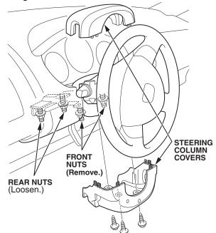
5. On Civics, disconnect the 16P connector from the combination light switch and the 5P connector from the cable reel. On Civic Hatchbacks, also disconnect the 14P connector from the wiper switch. Then carefully pull the wire harness to the right of the steering column. On Insights, disconnect the 16P connector from the combination light switch.
