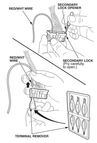
13. Twist off a terminal remover from the Terminal Remover Set (T/N 070AZ-S5A-011). Insert the terminal remover into the center row cavity of the 16P connector, above the RED/WHT wire cavity, then remove and discard the RED/WHT wire. 14. Strip off 7 mm of insulation from the vehicle wire harness side of the RED/WHT wire. Insert the stripped end into one side of the splice connector, and crimp the connector.
