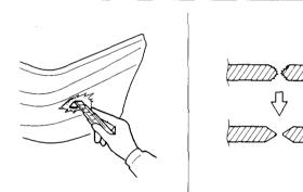
2. Air blowing/degreasing Clean the damaged area throughly.
