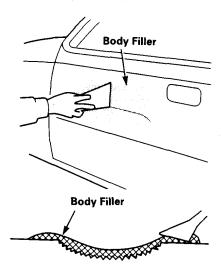
After applying the body filler, allow 5~6 minutes of normal drying time, then force dry it with infrared lamps or other industrial dryer at 122°F(50°C) ~ 140°F (60°C).
